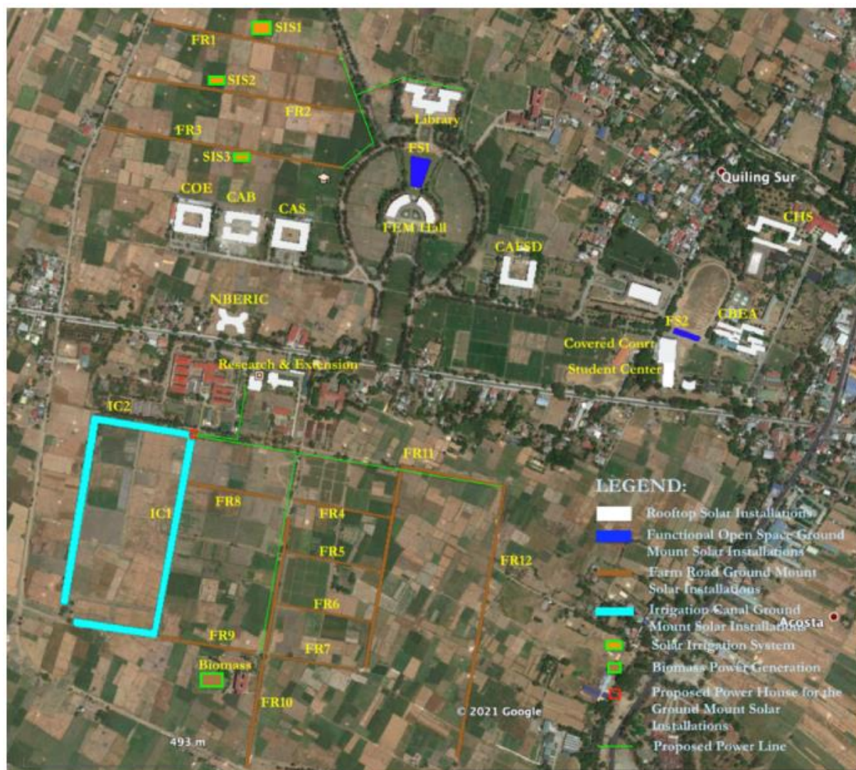
Fig. 2.1. MMSU NZEB site development plan showing the locations of each of the proposed renewable energy sources installations.
