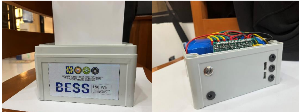
Figure 17. Developed Battery Energy Storage System (BESS)
